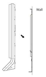
**4** Connect FaceStation F2 to the bracket by rotating the product fixing screw of FaceStation F2.
